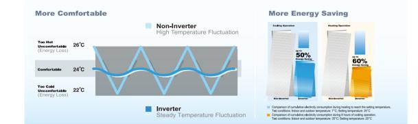
With MDV's Inverter technology, the air conditioner adjusts its power output to maintain the temperature precisely. When reaching the set temperature, the air conditioner will adjust the compressor speed to maintain a low power operation. As a result, money saving comfort!
